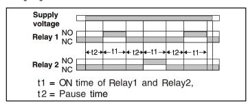
Forward - Pause - Reverse timer Special timer for repetitive forward and reverse motion of motor with intermediate pause timing.
