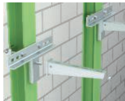
Clamp fastening on vertical steel girder Installation of the adapter plate, type KA-AW, on the vertical steel girder using clamping angle or chuck jaws. Wall brackets of type AW are fixed to the adapter plate, using the hexagonal bolt SKS 12 x 40 GF.
