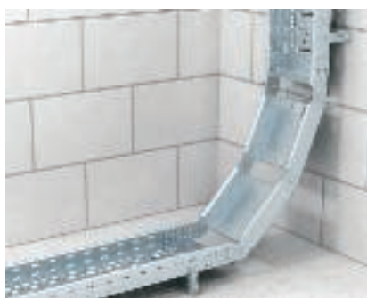
Installation of rising adjustable vertical bend Adjustable vertical bend to bridge height offsets or when changing from horizontal to vertical. The adjustable vertical bend is fastened to the cable tray directly using the adjustable connectors.
