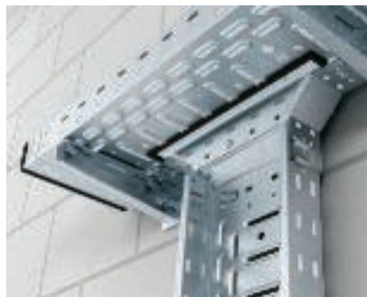
Mounting of Magic vertical mounting/branch piece (bottom view) Vertical mounting of the add-on tee as length-wise funnel. Perforation in the cable tray is created on site. For widths > 400 mm, please order connectors separately.
