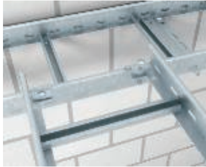
Installation of tee Creation of a horizontal tee exit of two cable ladders at different heights. The support angle, type LAW, is required to fix two cable ladders.
