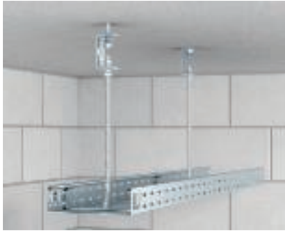
Centre suspension application Direct centre suspension with threaded rod, type 2078/M10. This mounting variant is possible for RKS cable trays of width 50 to 200 mm.
