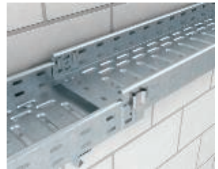
Straight connection, cable tray interconnection The ongoing cable tray is inserted from above from the existing sleeve opening.
