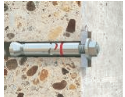
Heavy-duty anchor, type FH Heavy-duty anchor, type FH, with M12 threaded connection, for fixing components with large loads, approved for normal concrete C20/25 to C50/60. Load capacity 8.26 kN, with European technical approval.
