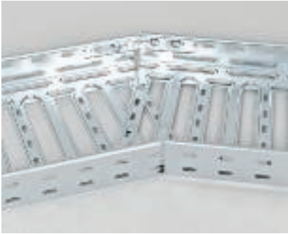
Horizontal angle connection of cable trays Step 3: After this step, place the two ends of the cable tray over one another and screw them to the base and the side rail. Appropriate angle connectors are required to screw on the side rail.
