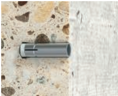
Impact tie type FZEA Impact tie, type FZEA, with M8, M10, M12 internal thread. For acceptance of smaller loads, approved for normal concrete C20/25 to C50/60. Load capacity 3.0 kN (M8) and 3.6 kN (M10 and M12). Suitable for function maintenance.
