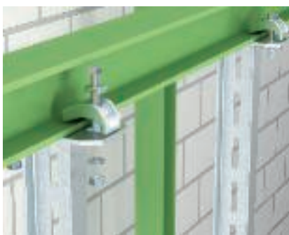
Direct girder clamping Direct girder clamping of an I support using chuck jaw (heavy-duty), type TKS-S-30. Route along steel girder.
