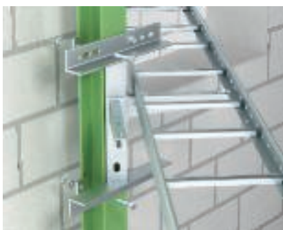
45° adapter plate, steel clamping Installation of the 45° adapter plate, type KA-E 45, on the steel girder using clamping angles or chuck jaws. For additional support of trays at room corners.
