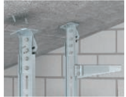
Head plate, variable (rotated through 90°) Installation of the variable head plate, rotated through 90°, KI 8 VLK to sloping concrete ceilings using anchor bolts, type FAZ II.
