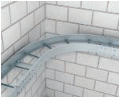
Installation of 90° bend Bend in combination with wide span cable ladder. The bend is connected to the wide span cable ladder using external connectors.
