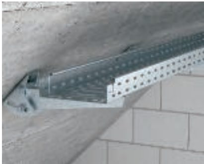
Wall bracket, variable Fastening of the variable wall bracket, type AWW, with anchor bolt, type FAZ II, to vaulted or sloping walls/ceilings.
