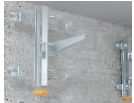
Wall mounting, I support Installation of an I support on the wall using mounting angle, type BW 80/55, and anchor bolts, type FAZ II, to accept multiple support brackets, type AS.
