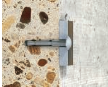
Anchor, type FNA, with drive-in head Nail anchor, type FNA, with drive-in head, usable in reinforced or unreinforced concrete C20/25 to C50/60, load capacity 0.5 kN. Suitable for function maintenance.
