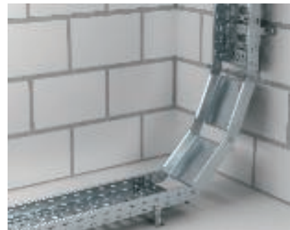
Installation of rising adjustable vertical bend Adjustable vertical bend to bridge height offsets. The adjustable vertical bend is connected with to the cable tray using the adjustable connectors.
