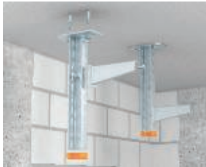
Standard mounting of support with wall bracket, single-sided without spacer Ceiling fastening of a support with single-sided bracket fastening. No spacer is required for widths up to and including 300 mm.
