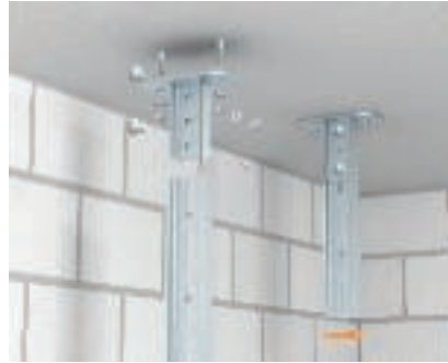
Head plate mounting Fastening of the standard head plate, KI 8, for I support to concrete ceilings using anchor bolts, type FAZ II.
