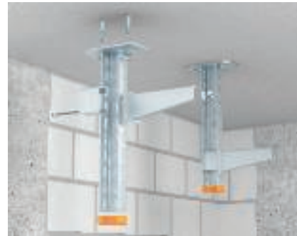
Standard mounting of support with wall and support bracket, single-sided with spacer Ceiling fastening of a support with single-sided bracket fastening. For widths of over 400 mm, we recommend using a spacer.
