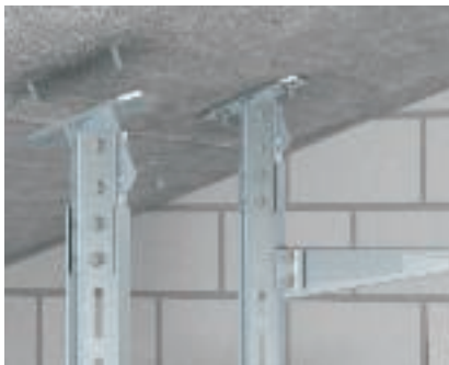
Variable head plate Installation of the variable head plate KI 8 VQP to sloping concrete ceilings using anchor bolts, type FAZ II.
