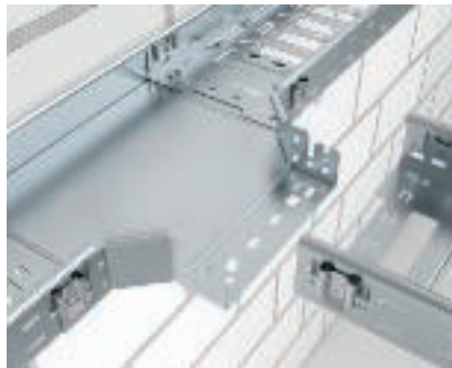
Mounting of Magic T branch piece Mounting of fittings by simple interconnection. For this, the cable tray with the spring side is locked into the fitting connection from above.
