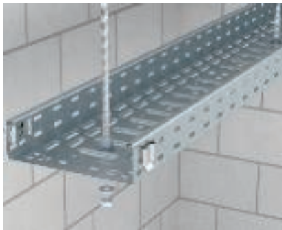
Centre suspension with threaded rod Direct centre suspension at low loads of a cable tray with threaded rod 2078/M10.
