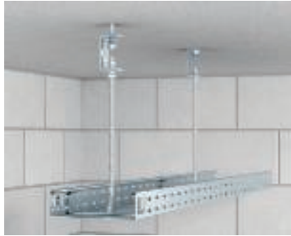
Installation of centre suspension Installation of the central suspension MAH 60 on the ceiling using threaded rod 2078/M10 and ceiling bracket 12050. Maximum cable tray width 300 mm.
