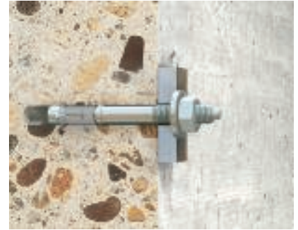
Anchor bolt, type FAZ II Anchor bolt, type FAZ II, for fixing heavy-duty anchorings in reinforced or unreinforced normal concrete C20/25 to C50/60, suitable for push-through mounting, with M8, M10 or M12 connection thread. Load capacity 4.3 kN (M8), 7.6 kN (M10), 11.9 kN (M12). With European technical approval. Suitable for function maintenance.
