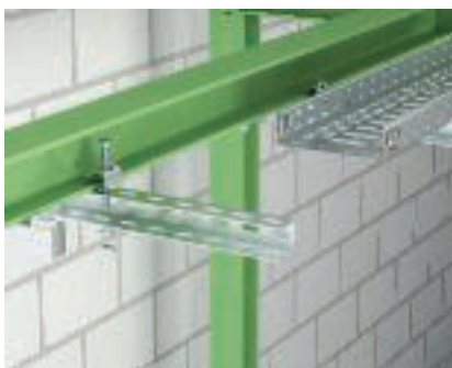
Cantilever beam on steel Installation of U support as cantilever beam on steel girder. Fastening with clamping angles or chuck jaws depending on load. Fastening with spacers, type DSK.
