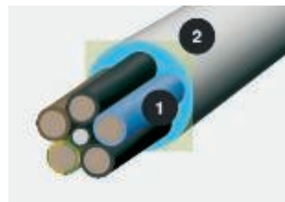
Cable diameter (1) and space required (2)
