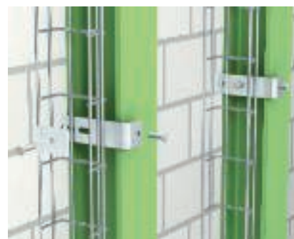
Vertical clamp fastening Installation of a mesh cable tray vertically on a steel girder, mounting with a beam clamp BFK and clamp GKS 50.
