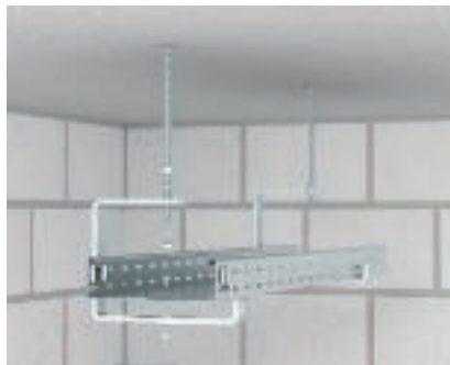
Threaded rod suspension with ceiling bracket Ceiling mounting of a cable tray with AHB ceiling bracket and threaded rod 2078/M10. Maximum cable tray width 400 mm.
