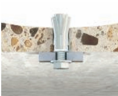
Hollow ceiling tie Hollow ceiling tie, type FHY, with internal thread M8, M10. For use in pre-stressed concrete core slab ceilings. Load capacity 2.0 kN (M8) and 3.0 kN (M10). Approved for function maintenance.
