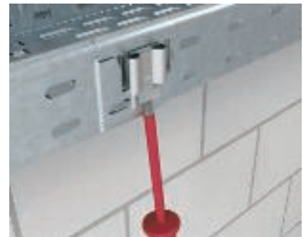
Slackening the connection Of course the connection can be loosened again. To do this, simply push a screwdriver under the spring element. This releases the lock function.
