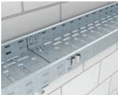
Straight connection, cable tray interconnection The optimum straight connection is confirmed by an audible click. Then use a screwdriver, to turn over the connection lugs in the bottom – and you're done!
