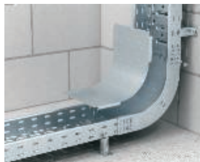
90° bend (rising/falling) The 90° vertical bend is pushed over the rail of the cable tray and bolted with truss-head bolts, FRSB M6x12 mm. The cover is placed on loosely and fastened using the incoming cable tray lid. The cover clamp DKU can be used for additional fastening.
