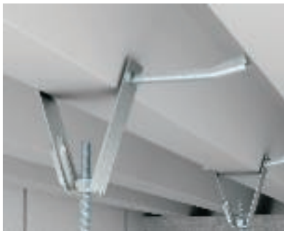
Installation of trapeze suspension Installation of a cable tray on a trapezoidal ceiling using a ceiling bracket, type TPB 100 and central suspension, type MAH 60. Maximum cable tray width 300 mm. The trapezoidal fastening is mounted using the lock, type TPB R.
