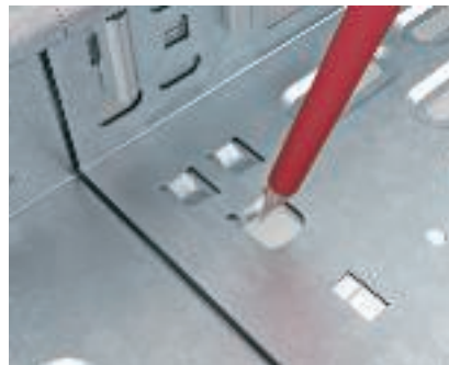
Straight connection, cable tray interconnection It is possible to turn over the connection flap in the floor of the cable tray using a normal screwdriver.
