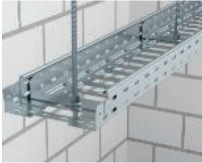
Centre suspension application Centre suspension of the cable tray systems MKSM, SKSM and IKSM with a central hanger, type MAH, and threaded rod 2078/M10.
