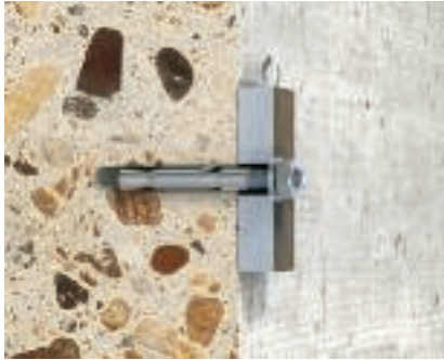
Anchor, type FNA, with threaded connection Nail anchor, type FNA, with M8 threaded connection, usable in reinforced or unreinforced concrete C20/25 to C50/60, load capacity 0.5 kN. Suitable for function maintenance.
