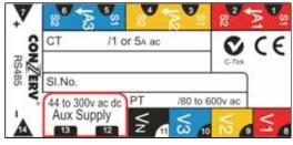
Terminals are numbered, coloured and grouped such that defect free wiring is ensured.
