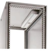
**Description:** Fluorescent lamp equipped with switch electronic starter integrated socket and a protection cap. A male GST 18/3 connector is provided for connection to the power on one side and by a pass-through circuit to a female connector allows a further connection on the other side. An additional connector ST 17/2 allows the activation of the lamp by a doorswitch. **Power:** Standard socket:120/230 V/ 50/60Hz / 16A Schuko. Other country specific sockets available on request.
