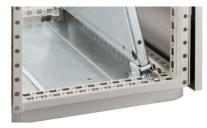
**Description:** With these brackets the mounting plate can be adjusted in depth by steps of 25 mm in the enclosure frame. **Material:** 3 mm zinc plated steel. **Pack. quantity:** 2 brackets with mounting material.
