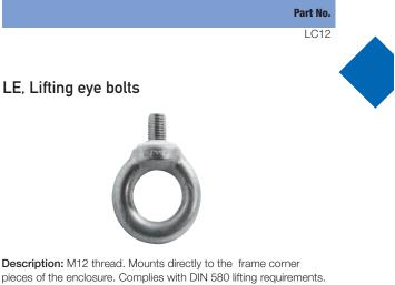
pieces of the enclosure. Complies with DIN 580 lifting requirements. Maximum load: 3400N per lifting eye with max angle of 45°. Please follow Eldon lifting instructions. Pack. quantity: 2 pieces
