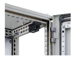
**Description:** Activates any electrical device (lighting, coolers, etc.). Can be fitted after installing the enclosure thereby keeping the door opening free. Fixed (without screws) on the inside hole pattern of the enclosure frame. Cable entry M 20.
