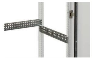
Description: Universal profile for both depth and width fitting on the 25 mm DIN hole pattern of the enclosure frame or in combination with the VB profiles. The 75 mm wide profile is equipped with three rows of holes of which one is turned 90 degrees. This makes it possible to mount the CLPF profiles in both directions. The CLPK can be secured by the use of self tapping screws. Material: 1.5 mm zinc plated steel.
