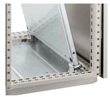
**Description:** Standard mounting plate. Fixing bracket kit MPA 06 to be ordered separately. Can also be mounted in the side of an enclosure by using bracket kit MPS or slide in from the side by using the sliding profile MTS. For heavy loads in vibrating environments use mounting plate reinforcement profile MPR and MPE or MPEF brackets.
