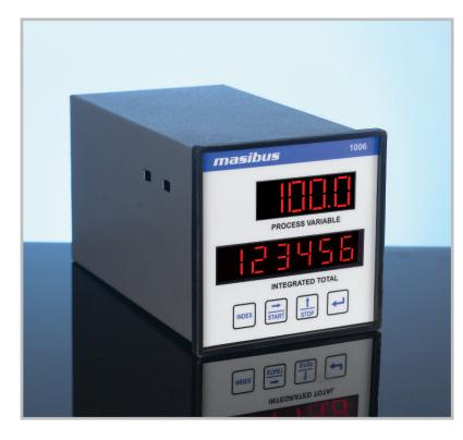
Masibus' Model 1006 is a panel mounted rate totalizer with separate rate and total displays. When connected with a 4/20mA flow transmitter, Model 1006 will display the rate of flow in engineering unit and total flow in the same or different engineering unit. If the loop is disconnected or auxiliary power fail, the displayed total and all programming parameters are stored in non-volatile memory, and are automatically recovered when the loop/auxiliary power is restored.
