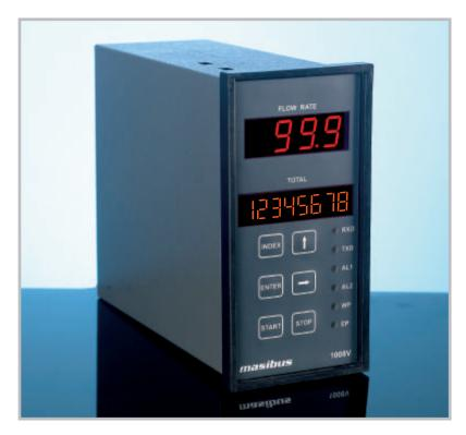
Masibus' Model 1008V is a panel mounted high precision rate totalizer with separate rate and total displays. When connected with a 4/20mA flow transmitter, 1008V will display the rate of flow in engineering unit and total flow in the same or a different engineering unit. If the loop is disconnected or auxiliary power fail, the displayed total and all programming parameters are stored in non-volatile memory, and are automatically recovered when the loop/auxiliary power is restored.
