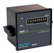
The energy meter has six moving counters and three static or fixed zeros. For example if the meter reads the energy value as 123456 000, 123456 are the six moving counters and the remaining are the three static zeroes.
