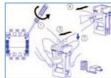
Contact replacement ( \geq 100A )
