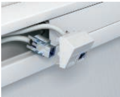
Device installation in data technology support Insert the complete data technology connection module into the data technology support from behind. For this, insert the support plate of the connection module into the seat and lock it in place.
