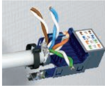
Device connection – strain relief Attach the cable to the cable seat and relieve the strain using the enclosed cable ties. With shielded cables, ensure that the contacting strap is connected to the shield.
