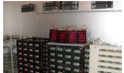
Burn-In at 55°C to Ensure Stability
