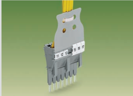
Removable terminal block module with CAGE CLAMP® connection (0.25 mm 2 – 2.5 mm 2 / AWG 24 – 14), with strain relief plate and marker position for miniature WSB or WMB marking.
