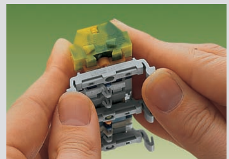
Terminal strip with snap-in mounting feet, assembly of mounting adapter 209-120 1) 1) The distance between mounting adapters should be 35 - 40 mm / 1.378 - 1.575 in max.
