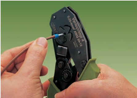
Introduce conductor with ferrule into crimping station.
