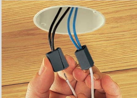
To connect: Press button fully and insert stripped conductor into square entry and release
