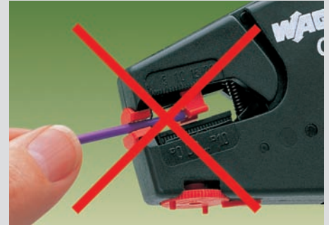
FIT CLAMP connection without stripping
