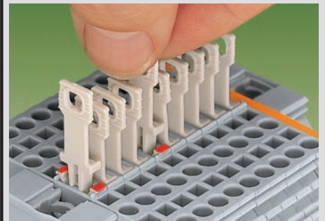
Pulling the disconnect tab by hand
