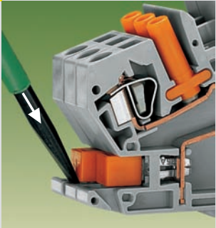
Insertion of insulated, touchproof adjacent jumpers into the protected shorting position
