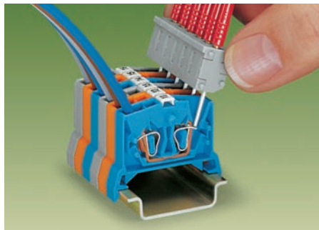
Testing with touch contact at the CAGE CLAMP® connection made of spring steel – limited to a current of 0.5 A max.
