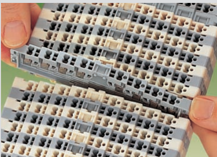
. . . move terminal block laterally and remove from the rail with a levering action
