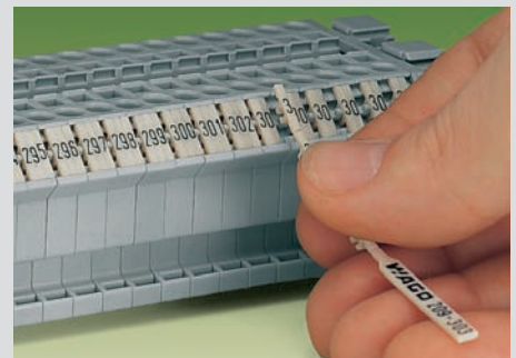
Snapping markers into the marker receptacle profile up to 2 branch markers, series 279 up to 3 branch markers, series 280 to 285
