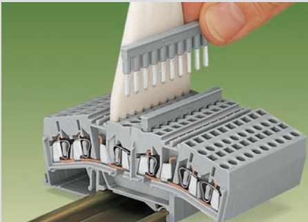
Used as potential multiplication. Insertion of a 10-way comb type jumper bar (only possible in the center)
