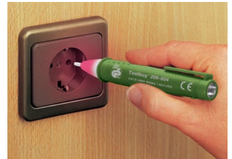
A device that will reliably detect A.C. voltages in cables, sockets, fuses, switches, connector boxes, etc.
